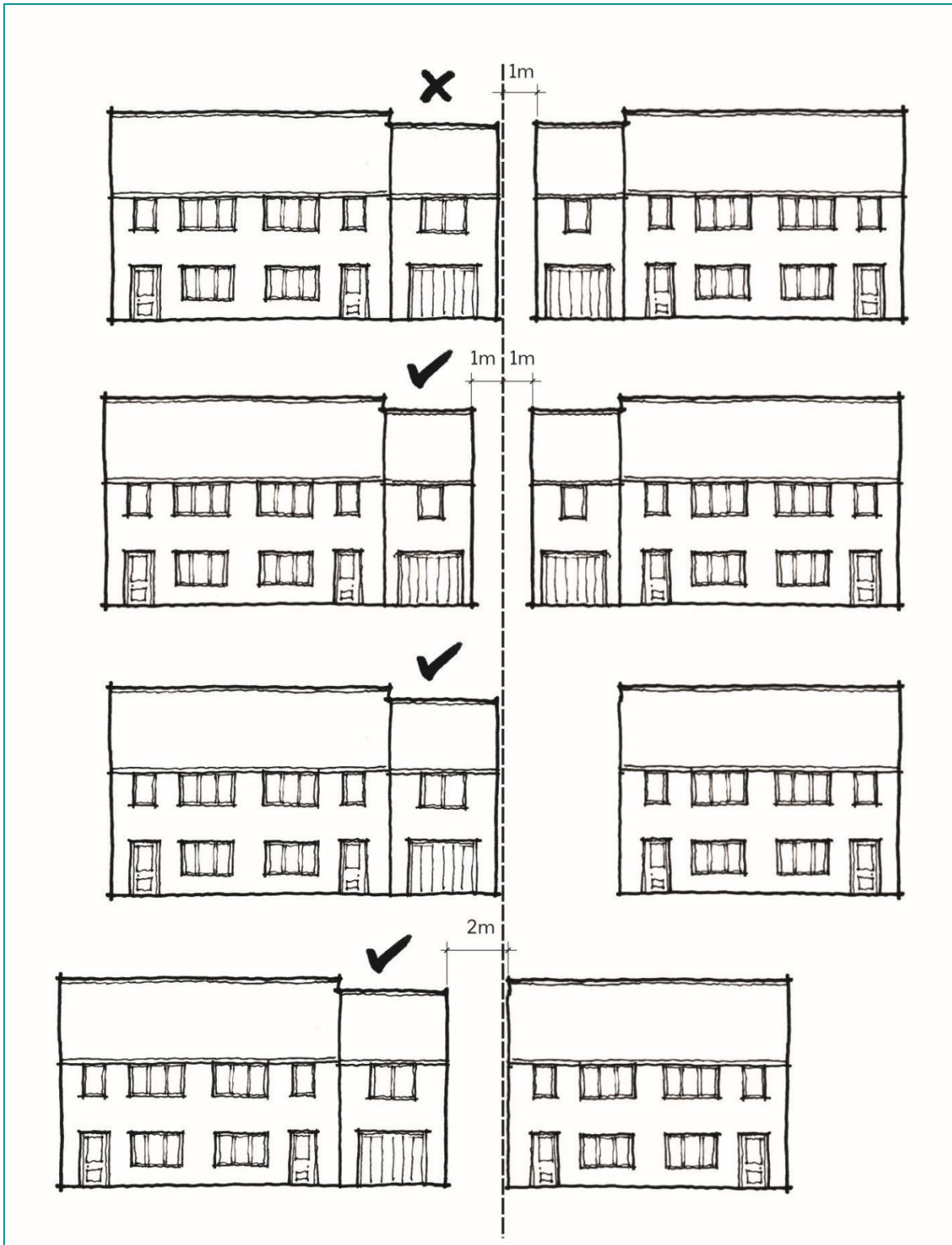
Fig.2 - shows side extensions designed to avoid the 'terracing effect'.
